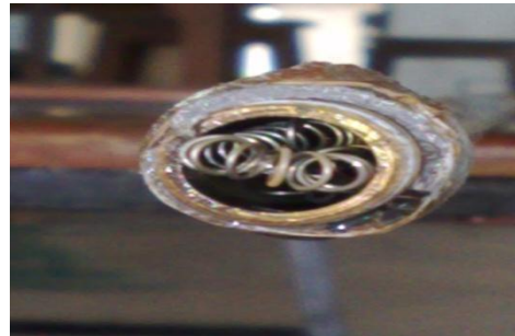
Fig 3: Inner tube with turbulators
